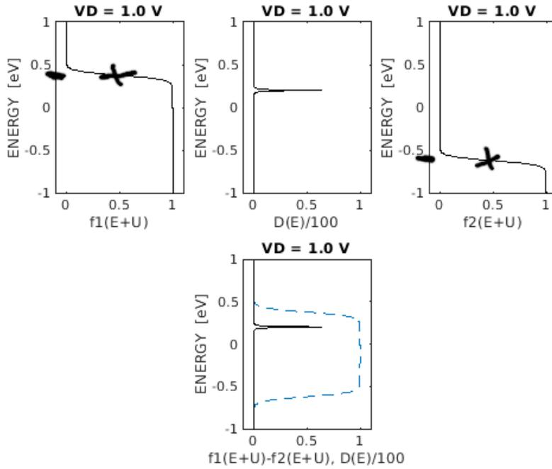
Figure 3: Marked step points of contact Fermi functions.
